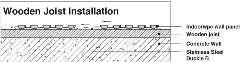
**Note: Use iron joist or wood joist to do the wall leveling job, keep as installation foundation. Fix the first piece of great wall panel on the joist, insert the stainless steel buckle B at wall panel's side, then install the next piece of great wall panel.**
